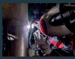
Alternatively, 33 minutes of continuous TIG welding can be performed (at 100 A)
