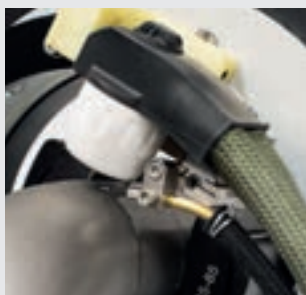
/ Wire feeding, torch bracket from 0 - 45° stepless swivelling
