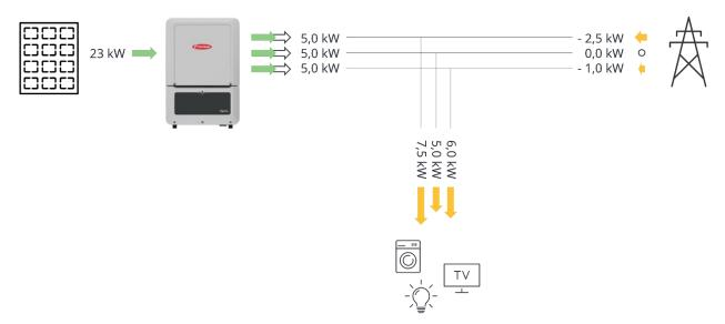
With the introduction of asymmetrical generation, it's now possible to precisely match the production to the demand on each phase while still ensuring zero physical feed-in.
