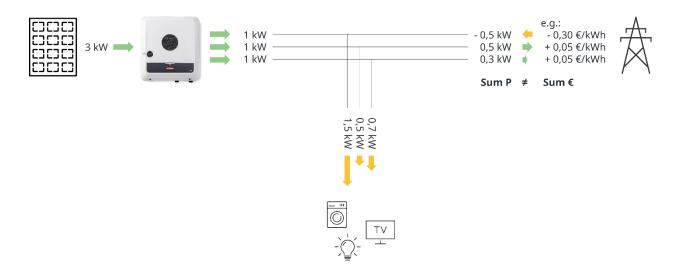
Example of Symo GEN24 10.0 Plus incl. Battery with <u>symmetric</u> generation and feed-in limitation of 7 kW: In night-hours, energy is exported to the grid on certain phases and consumed on other phases, while the sum of the energy flows remains zero. In day-hours, feed-in to the grid is limited with 7 kW in total, but exceeds 2,33 kW (33% of 7kW) on some phases as a result of household load asymmetry.
