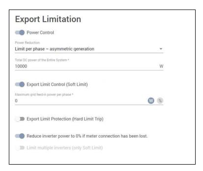
Example for "Asymmetric Generation" with Zero-grid feed-in limitation. In this case, the inverter will generate asymmetric power to reduce grid consumption, and also avoid any power export to the grid.
