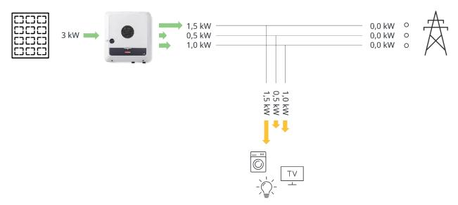
Example of Symo GEN24 10.0 Plus incl. battery with <u>a</u>symmetric generation and 2,33 kW feed-in limitation per phase: In night-hours, energy consumption from the grid is prevented efficiently and household loads are covered by the battery. In day-hours any feed-in to the grid is limited with 2,33 kW per phase (7 kW in total) and the inverter pushes its production towards this limit by compensating household loads with asymmetric generation.
